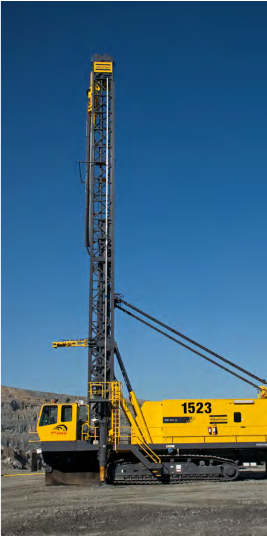
Boliden undertook a thorough evaluation before deciding to invest in four new Pit Viper 351E rotary drill rigs. Boliden's criteria included the ability to drill 311 mm holes to a depth of 19 meter. In addition they looked for safety and productivity enhancing features.
