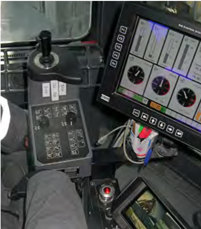
The PV-351 could offer features like finger-tip joystick controls, a comfortable cabin, ability to drill angled holes, and ease of raising and lowering the tower for tramping.
