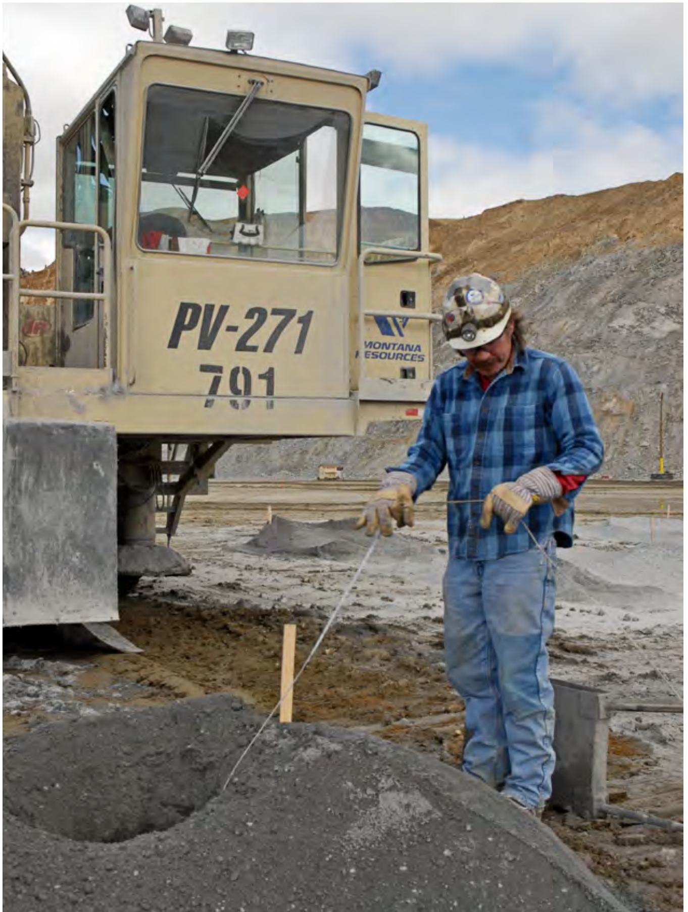
Brian Lankford takes measurements of a 9 7/8-inch hole to 28 feet deep.
